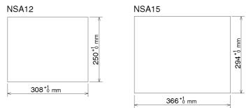
2. Insert the NSA-series Industrial PC into the hole from the front of the panel.
