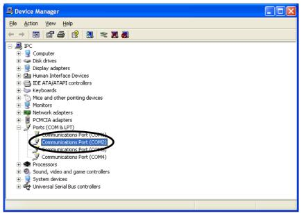
Note: COM3 and COM4 are used by the NSA-series Industrial PC system internally. Do not select these ports.
