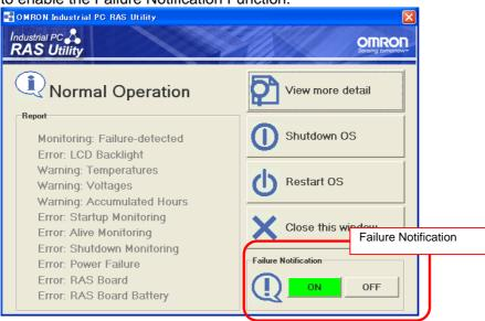
The icon shows the status of the Failure Notification Function.
