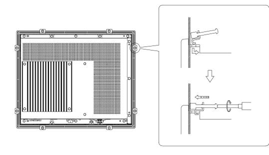
• The mounting panel must be between 1.6 and 4.0 mm thick.
