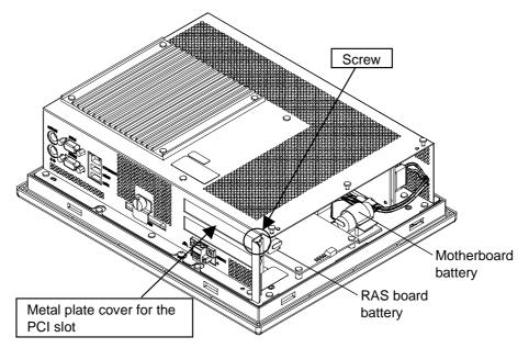
2. Insert the PCI Board into the PCI Board mounting connector.
