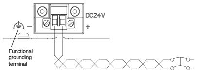
Attach a crimp terminal for an M4 screw to the grounding wire.
