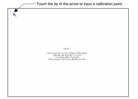
5. After all the calibration points have been entered, the Check calibration dialog box will appear. A message will be displayed prompting you to save the calibration data. If there were no problems with the calibration points, press the OK Button or the Enter Key on the keyboard. If there was a problem with a calibration point, do not touch anything for 10 seconds. The calibration data will be discarded and will not be saved.
