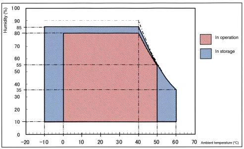
■ Note 2: Use the temperature and humidity ranges in the following diagram.
