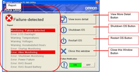
Note: For details on using this window, refer to the RAS Utility's Help function.
