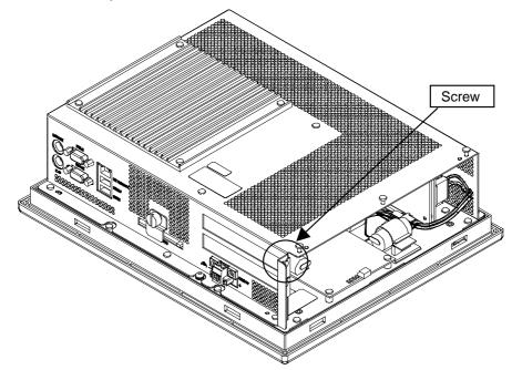
3. Secure the PCI Board with the screw that was removed from the metal plate cover in step 2.
