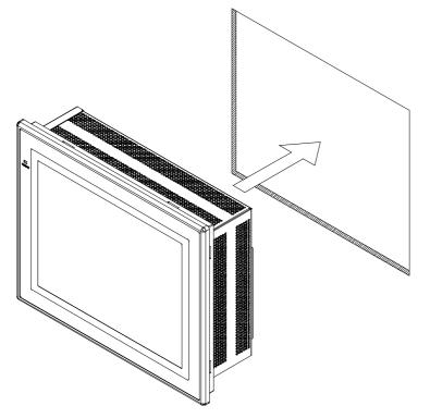
Use the Mounting Brackets provided to secure the NSA-series Industrial PC in the panel. Tighten the Mounting Brackets evenly to the specified torque. Failure to do so may cause the front sheet to buckle.
