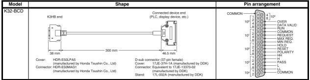
Note: The BCD Output Cable has a D-sub plug. Cover: 17JE-37H-1A (manufactured by DDK); Connector: equivalent to 17JE-23370-02 (D1) (manufactured by DDK)
