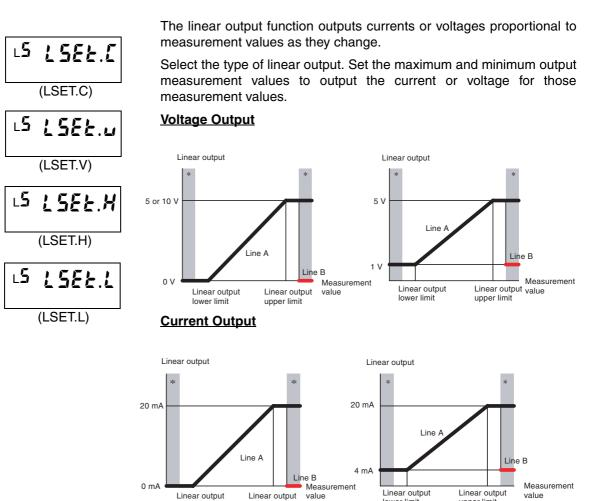
\* Areas marked with an asterisk (\*) are input error areas. If the "operation at input error" parameter is set to "input error," then the output would be like Line B. Otherwise, the output would be like Line A.
