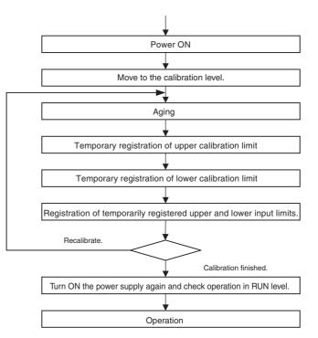
The input type that can be calibrated according to this flowchart is the type selected under the "input type A" parameter. To calibrate other input types, switch the setting for input type A in the initial setting level to the desired input type and then perform calibration according to the flowchart outlined above.
