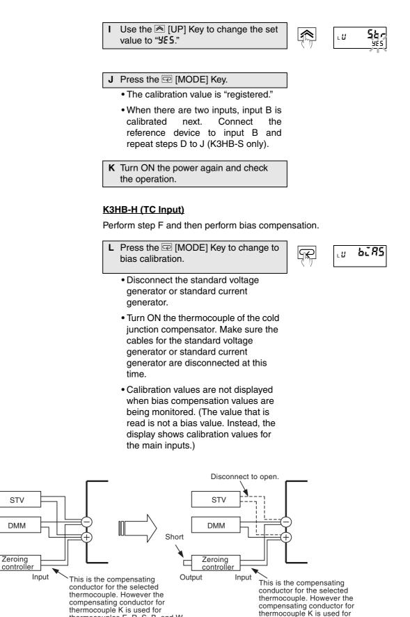
thermocouples E, R, S, B, and W.
