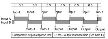
\* The output every 0.5 ms is the comparative output corresponding to the input change for either input A or input B. The input change for both inputs is reflected in the comparative outputs every 1 ms.
