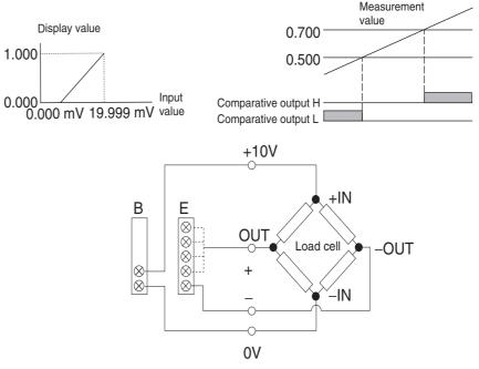
\* 2 mV/V indicates a load cell output of 2 mV for 1 V applied voltage for the rated load (when using a load of 1 N). When the applied voltage is 10 V, the load cell output is 20 mV (2 mV×10)
