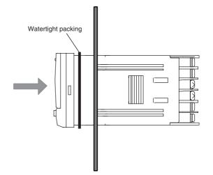
(3) Insert the adapter into the grooves on the left and right sides of the rear case and push until it reaches the panel and is fixed in place.
