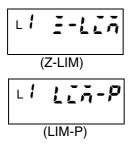
Set the following parameter for zero-limit. The zero-limit value can be set only when zero-limit has been enabled.
