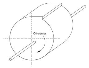
As shown in the above diagram, when rotating a cylindrical object and measuring the distance from the object using a laser displacement meter, it cannot be judged if the increase in measurement values when the rotating axis is eccentric is due to the eccentricity or to a burr.
