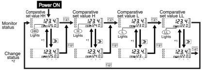
\*1 If no key is pressed for 5 seconds, the set value is registered and the display returns to monitor status. \*2 Use the 🔊 [SHIFT] and 🗟 [UP] Keys to set the set value.
