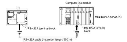
**Note:** When connecting to a terminal block, always use crimp terminals.
