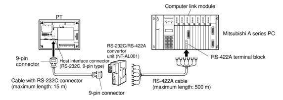
⚠ Caution: After connecting a communication cable, always secure it with the screws.
