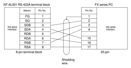
Make the connections between SDB and SDA, RDB and RDA, and RSB and RSA, with twisted pair wires.
