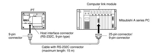
Caution: After connecting a communication cable, always secure it with the screws. Otherwise the cable may disconnect, causing operation to fail.
