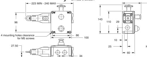
Note: The designation of the ER1022 switch as left-sided or right-sided is based upon the mounted position of the switch, in the installation.
