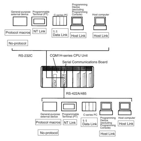
Note An NT-AL001-E Converting Link Adapter can be used to convert between RS-232C and RS-422A/485. This Link Adapter requires a 5-V power supply. Power is provided by the RS-232C port on the Serial Communications Board when the Link Adapter is connected to it, but must be provided separately when connecting the Link Adapter to other devices.
