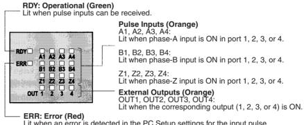
Lit when an error is detected in the PC Setup settings for the input pulse function, or when an overflow or underflow occurs in the high-speed counter's present value.
