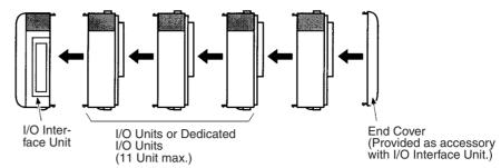
There is no Backplane for the CQM1H. The PC is constructed by connecting Units together using the connectors on the sides.
