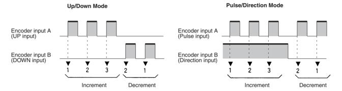
**Note** The function of encoder inputs A and B in Pulse/Direction Mode and Up/Down Mode differs from the Pulse I/O Board (CQM1H-PLB21).
