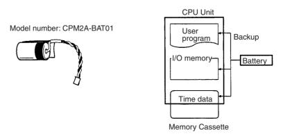
**Note** Do not remove the battery except when replacing it. If the battery is not replaced within 5 minutes after removal, internal data may be lost. For details on the replacement method, refer to *9-1 Battery Replacement*.
