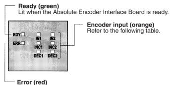
Lit when there is an error in the PC Setup for the Absolute Encoder Interface Board.
