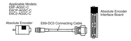
Applicable Cable: E69-DC5 Absolute Encoder Interface Board Connecting Cable (length: 5 m)
