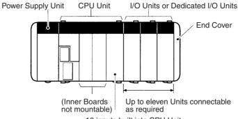
16 inputs built into CPU Unit
