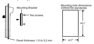
Allow at least 80 mm for the cable connector above the Programming Console.
