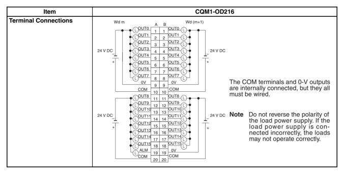
Note If the output current of any output exceeds the detection current, the output will be turned OFF. At the same time, the alarm output (ALM) will turn ON (Low).
