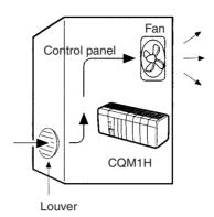
The ambient temperature range in which the CQM1H can be used is 0 to 55°C (0 to 45°C if a Programming Console is connected to the CPU Unit).
