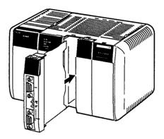
Caution Always turn the power OFF before installing or removing the Inner Board. Installing or removing the Inner Board with the power ON can cause the CPU Unit to malfunction, damage internal components, or cause communications errors.
