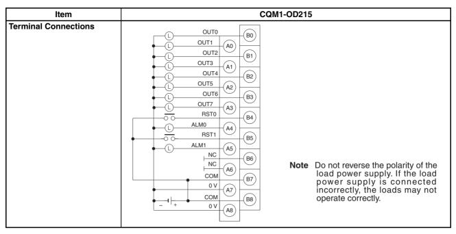
**Note** If the output current of any output exceeds the detection current, the outputs will be turned OFF at the four points (OUT0 to 3 or OUT4 to 7) which include that output. At the same time, the alarm output (ALM0 or ALM 1) will turn ON and the alarm indicator will light.
