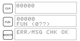
5. Press the CLR Key to bring up the initial programming display (program address 00000). The new program can be written at this point.
