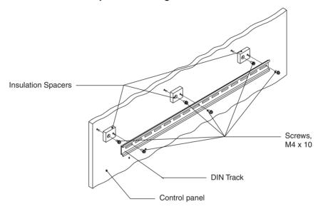
First connect the Insulation Spacers to the control panel using screws and then mount the DIN Track to the Insulation Spacers.
