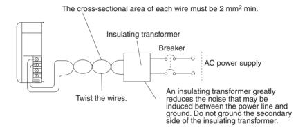
/ Caution Be sure that the AC power supply voltage remains within the allowable voltage range. For details refer to 2-1-1 Power Supply Units.
