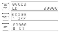
The cursor in the lower left corner of the display indicates that the force set is in progress. The bit will remain ON as long as the Set Key is held down.
