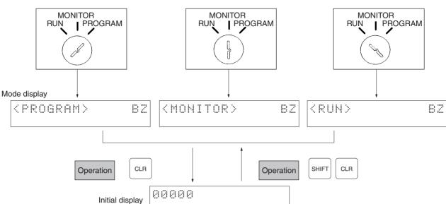
The CQM1H will enter RUN mode automatically if a Programming Console isn't connected when the CQM1H is turned ON.
