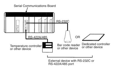
Both RS-232C and RS-422A/485 ports are provided. The RS-422A/485 port enables 1:N connections to general-purpose external devices without going through Converting Link Adapters. The 1:N connections can be used with protocol macros or 1:N-mode NT Links.
