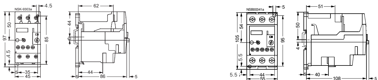
Figure 4-31: 3RU11 26-..B., 3RB10 26, (frame size S0) with terminal bracket for stand-alone installation
