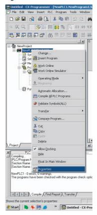
2. Select the *Execute Timer/Counter as Binary* Option in the PLC Properties Dialog Box. The timers and counters for all tasks will be executed in binary mode.
