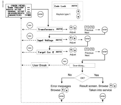
Figure 11: Auto setup of parameters.
