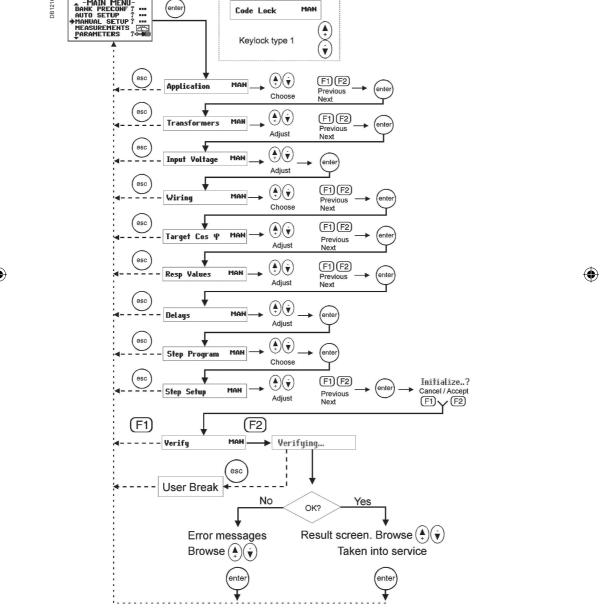
Figure 12: Manual setup of parameters.
