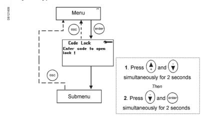
Figure 4: Entering a submenu with a keylock.
