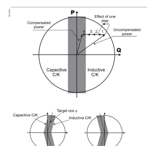
Figure 18: Compensation example and consequences.
