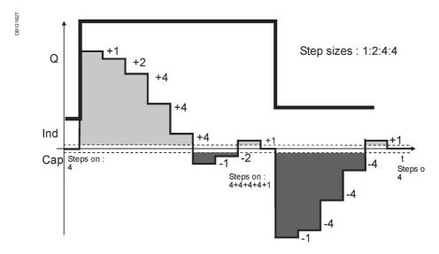
Figure 17: Regulation example - Optimal vs. Normal
