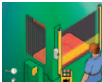
Defined PSDI window prevents unintentional cycle start due to reaching above or reaching below
