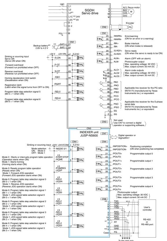
\*1: The L3 terminal is for specifications requiring a three-phase power supply. \*2: The control power supply for 400 V-class servo drive is 24 VDC.
