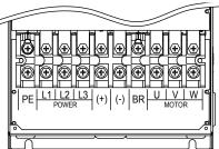
Frame 3 - Frame 7 supply and motor terminal
