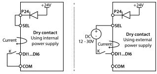
Figure 4-6 Dry contact connection
