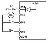
Figure 4-9 Connection when AC signal inputs (7.5 - 75kW)
