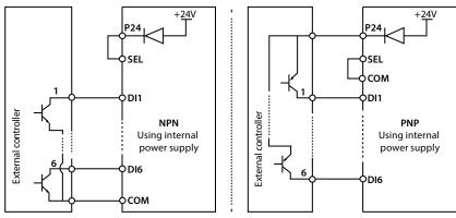
Figure 4-8 Connection when using internal 24V power supply
