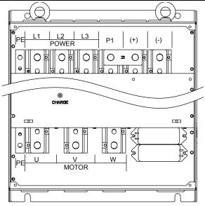
Frame 8 - Frame 11 / Frame 10 - Frame 11 (-C) supply and motor terminal
