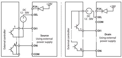
Figure 4-7 Source / Drain connection when using external power
