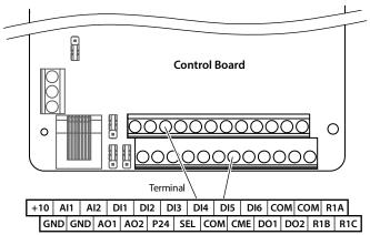
Figure 4-2 Control board terminal (90 - 400kW)
