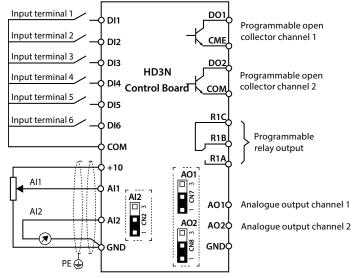
Figure 4-5 HD3N control board connection
