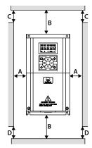
When one inverter is mounted on top of another, an air flow diverting plate should be fixed between them. Just as shown in Table 3-2.
