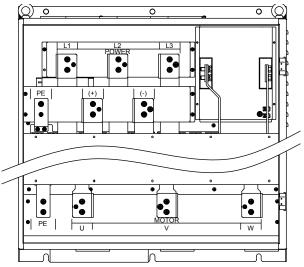
Frame 12 / Frame 12 (-C) supply and motor terminal
