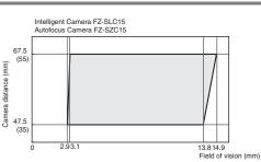
The value in parentheses is for the camera installation distance when using an Intelligent Camera.
