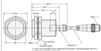
\*1.6-dia. vinyl-insulated round cable (flame retardant), Standard length; 300 mm
