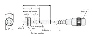
\*1. 4-dia. vinyl-insulated round cable (flame retardant), Standard length; 300 mm
