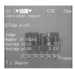
Connector pin-pitch inspection
