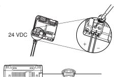
When you attach the ferrite core to the power supply cable, wrap the cable only one time.
