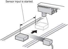
Trigger input sensor
