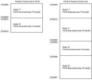
For the Position Control Unit, the areas are set only for node 17 (which has the first area for each of the three memory areas).
