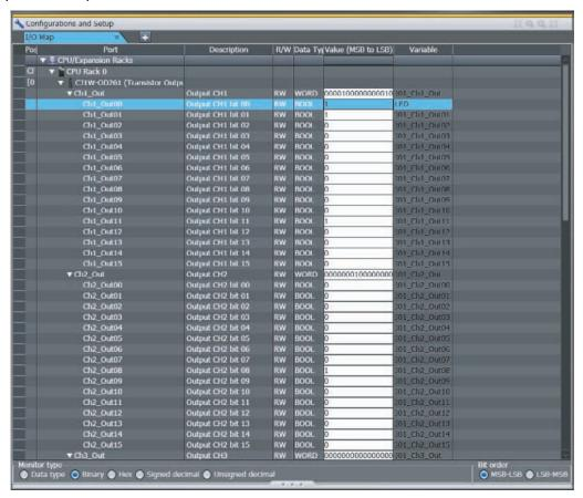
Right-click a slave or I/O port in the I/O map and select [Create Device Variable]. The device variable name is automatically created as a combination of the device name and the I/O port name. You can also select an I/O port and enter a variable name in the [Variable] column.
