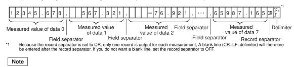
If data is output as an array for one output data, a field separator is inserted between consecutive array elements.
