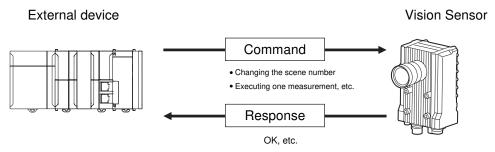
The external device sends a command as an ASCII string (e.g., "MEASURE" for a single measurement). The Vision Sensor then returns a response such as "OK", "NG", or some value.
