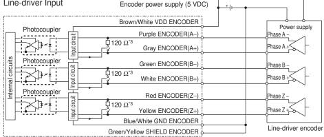
FQ-M \*3: The 120- $\Omega$  resistors are used when line driver encoders are connected. The terminating resistance can be turned ON and OFF from the PC Tool. Turn the terminating resistance ON or OFF according to the application conditions.
