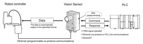
You can output commands to directly control a robot by combining text strings.
