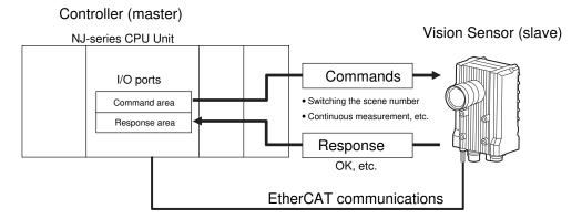
After you write a control command to an I/O port, such as Vision Command, you can turn ON the Control Command Execution (EXE) Bit to send the control command to the Vision Sensor via EtherCAT. The Vision Sensor executes the control command and sends a response back to the Controller via EtherCAT. The Controller stores the response in an I/O port, such as Vision Response.
