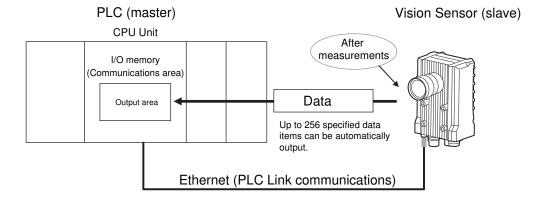
You must specify in advance the data to output after measurements. You must also specify in advance the Output Area in I/O memory to store the data in the PLC. After a single measurement or continuous measurements, the data is automatically stored in the Output Area of the PLC via Ethernet.
