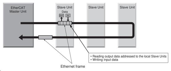
It is the "EtherCAT telegram" stored directly in an Ethernet frame that exchanges data regularly between the EtherCAT Master Unit and Slave Units.
