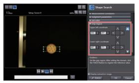
${\it 3}$  Specify the color of the workpiece in the gripping region and use it to teach the basic color area of the specified color. Refer to the below for instructions on how to specify the set color.
