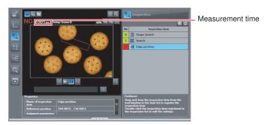
The measurement time is the time taken from when a trigger is input until when all measurement processes are executed.
