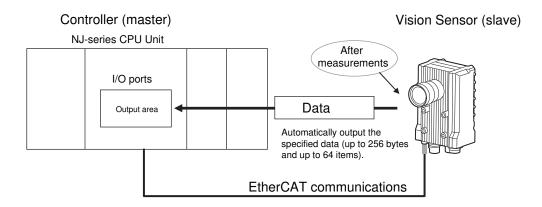
You must specify in advance the data to output after measurement is performed (up to 256 bytes and up to 64 items). After a single measurement or continuous measurements, the data is automatically stored in the I/O port in the Data Output Area of the Controller via EtherCAT.
