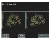
Displays the measurement results of all connected Sensors. Green display: OK, Red display: NG
