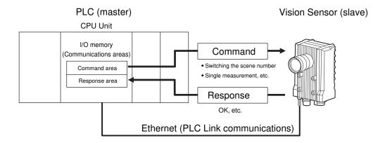
After you write a control command to the specified Command Area in the I/O memory of the PLC, you can turn ON the Command Execution (EXE) Bit to send the control command to the Vision Sensor via Ethernet. The Vision Sensor executes the control command and sends a response back to the PLC via Ethernet. The PLC stores the response in the specified Response Area in I/O memory.
