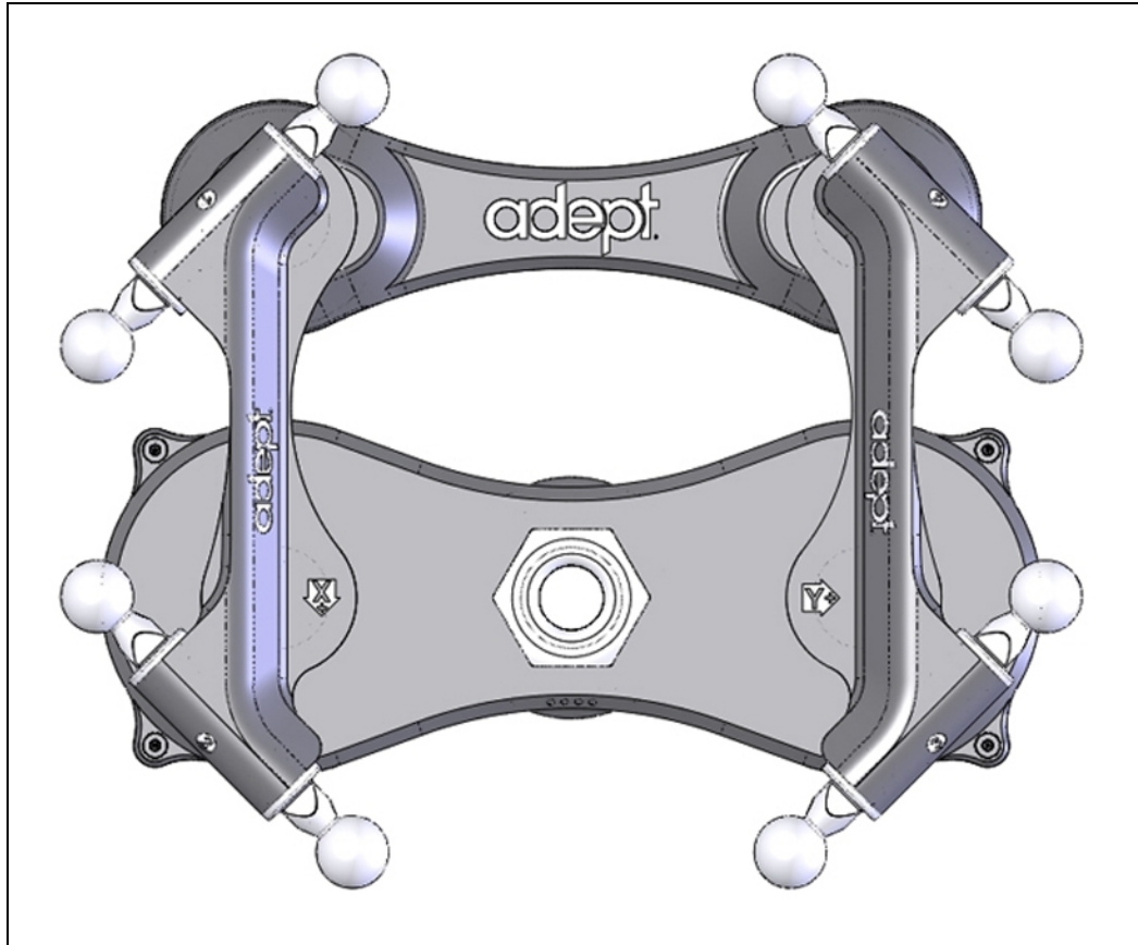
Figure 3-6. Platform Orientation Labeling (P34 shown)
