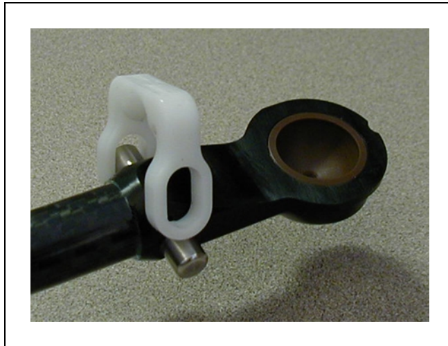
Figure 10-13. Horseshoe over One Pin, H Shown
