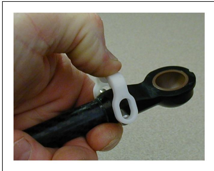
Figure 9-16. Squeezing the Horseshoe into Position
