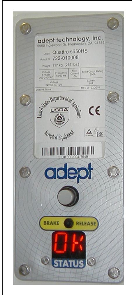
Figure 10-8. Status Display Panel, Showing 8 Hex-head Bolts
