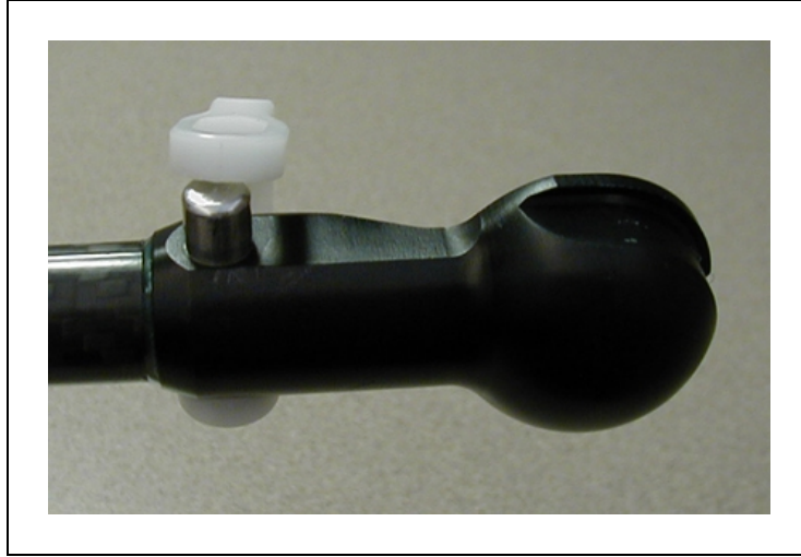
Figure 9-15. End of Horseshoe on Pin
