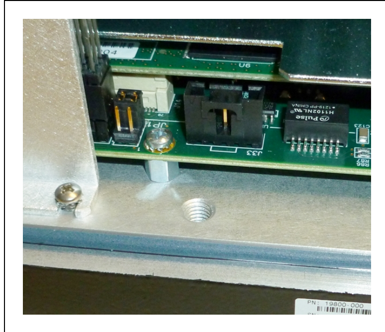
Figure 10-5. Ground Screw Hole on eAIB Chassis
