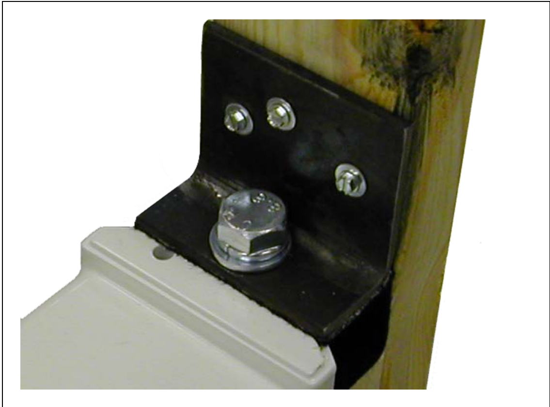
Figure 4-3. L-Bracket Securing Robot to Shipping Crate
