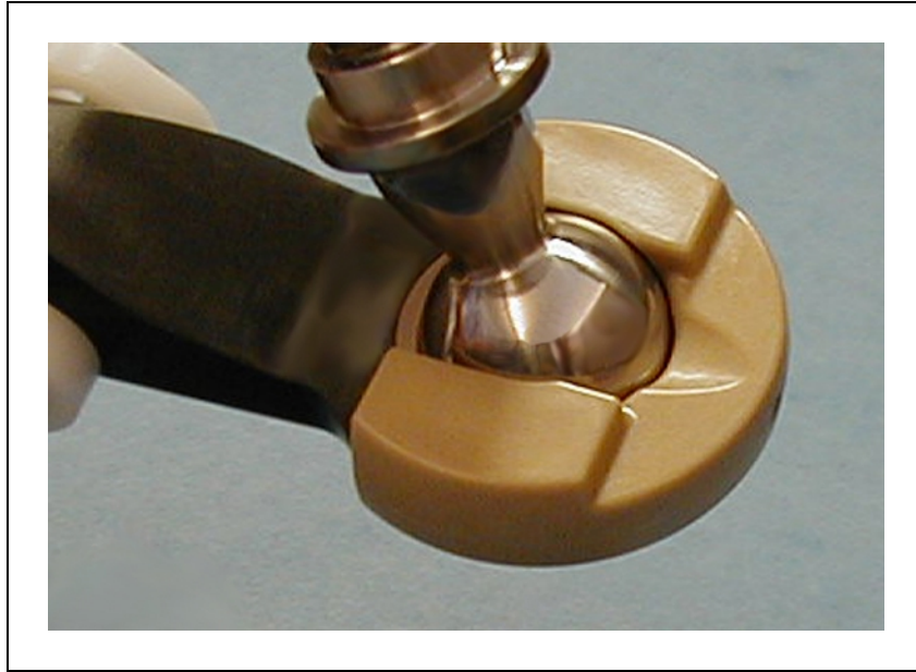
Figure 7-2. Ball Stud Lock on Ball Joint Socket
