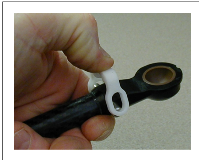
Figure 10-15. Squeezing the Horseshoe into Position, H Shown
