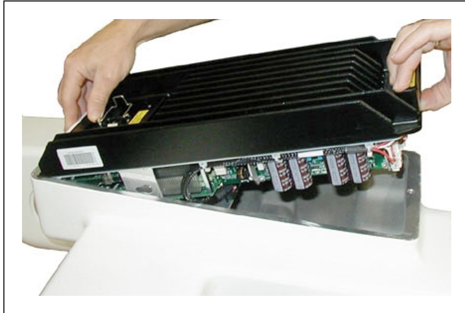
Figure 9-5. Opening the Chassis
