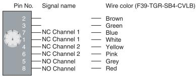
Note: If the auxiliary circuit is not fitted or not used then cut and discard the Yellow and Green Conductors.
