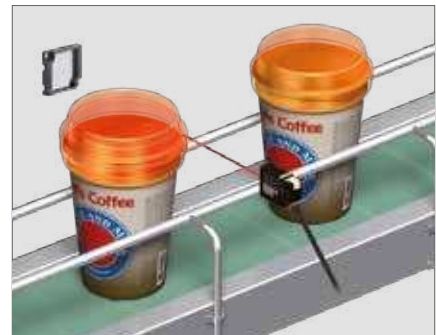
The small beam spot stably detects overlapping lids on cups.
