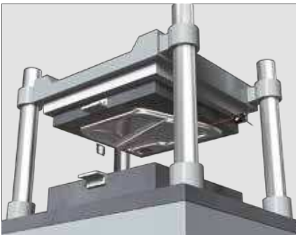
The small, long-distance spot can stably detect large pieces of sheet metal that remain on a press.
