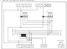
The "C" terminal blocks are short-circuited inside the controller.
