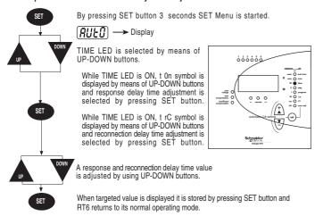
Note: Factory set values are 10 sec. for response delay and 50 sec. for reconnection delay
