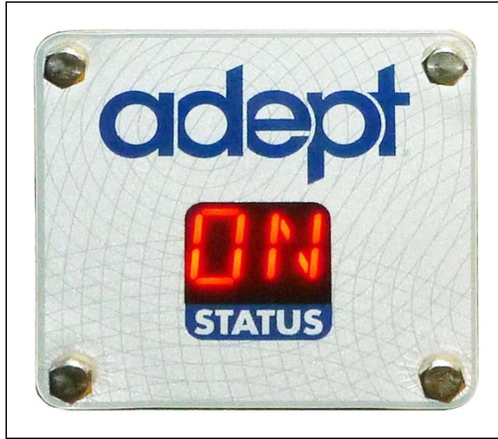
Figure 7-8. Status Display Panel Face
