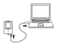
Use the exclusive cable to connect the Controller to the PC.
