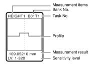
The currently measured profile is displayed. When multiple tasks are registered, switch the profile and display it for each individual task.
