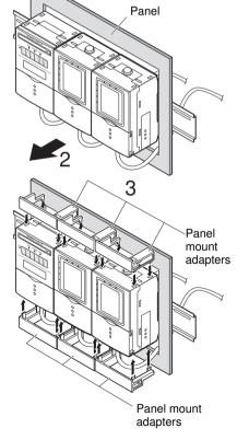
Install the short Panel Mount Adapters on the four holes on the Data Storage Unit and Controllers.
