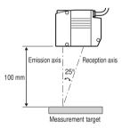
Mounting for diffuse reflection measurement
