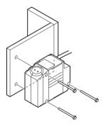
Fasten the Sensor Head onto the mounting base with M4 screws.
