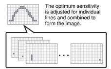
The amount of received light per individual line is judged and the appropriate sensitivity for each individual line is adjusted to accommodate for all kinds of shape, color and material. The measurement target must be made stationary as time is required to capture multiple image frames while changing the sensitivity.
