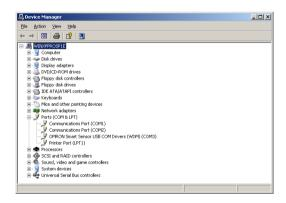
**3** Open [Ports (COM&LPT)] and check the COM number in "OMRON Smart Sensor USB COM Drivers (WDM) (COMxx)".
