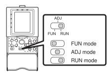
The ZG2-WDC has the following three operation modes. Switch to the desired mode before you start operation.
