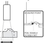
Set this level at a location where the target edge can be detected even if the measurement target moves horizontally.
