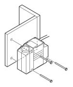
Fasten the Sensor Head onto the mounting base with M4 screws.
