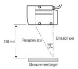
Mounting for diffuse reflection measurement
