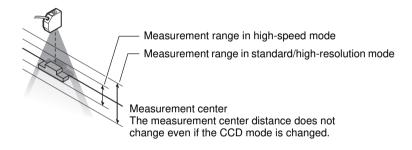
For actual details of measurement ranges, refer to the respective pages that explain mounting of each of the sensor heads.
