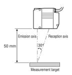
Mounting for diffuse reflection measurement
