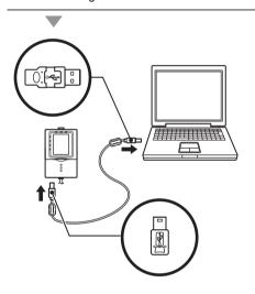
1 Connect the Controller to the PC with a USB cable.
