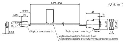
Note 1: Plug type connector The locking screws have metric screw threads (M2.6 x 0.45)
