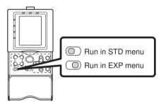
The STD and EXP menus are switched by the menu switch on the front of the Controller. The two menus cannot be selected simultaneously during menu operation as the menu is fixed by the menu switch.
