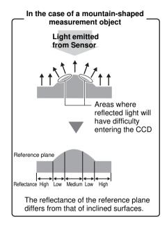
Areas having low reflectance cannot be measured due to insufficient light amount.
