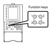
In the RUN mode, the following functions are assigned to function keys F1 to F4.
