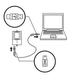
Use the USB cable provided with the ZG2-WDC□1A Controller to connect the Controller to the PC.
