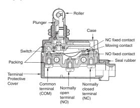
Note: M4 binding head screws (with toothed washers) are used as the terminal screws.
