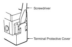
When mounting the Terminal Protective Cover to the case, align the cover on the case and then press the cover down to mount it firmly. If the cover is pressed down in an inclined position, rubber packing will deform and thus affect the sealing capability.
