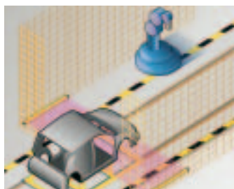
A horizontal light curtain without additional sensors and mechanics.
