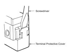
When mounting the Terminal Protective Cover to the case, align the cover on the case and then press the cover down to mount it firmly. If the cover is pressed down in an inclined position, rubber packing will deform and thus affect the sealing capability.
