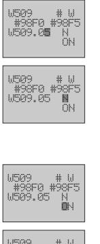
15. Use the Forward button to move the column cursor to the bit flag position. The present setting is the default setting.
