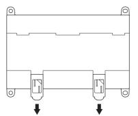
2. Lower the Units so that they catch on the top of the DIN Track, and then press them forward all the way to the DIN Track at the bottom.
