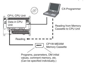
This function can be used for operations such as writing the required backup data to the CPU Unit for maintenance.
