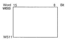
**Note** These words should be used first in programming be assigned to new functions in future versions of CP1L CPU Units.
