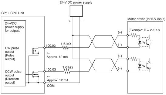
In this example, a 5-V input motor driver is used with a 24-VDC power supply. Be careful to ensure that the Position Control Unit output current does not damage the input circuit at the motor driver and yet is sufficient to turn it ON. Take into account the power derating for the 1.6-k $\Omega$  resistance.
