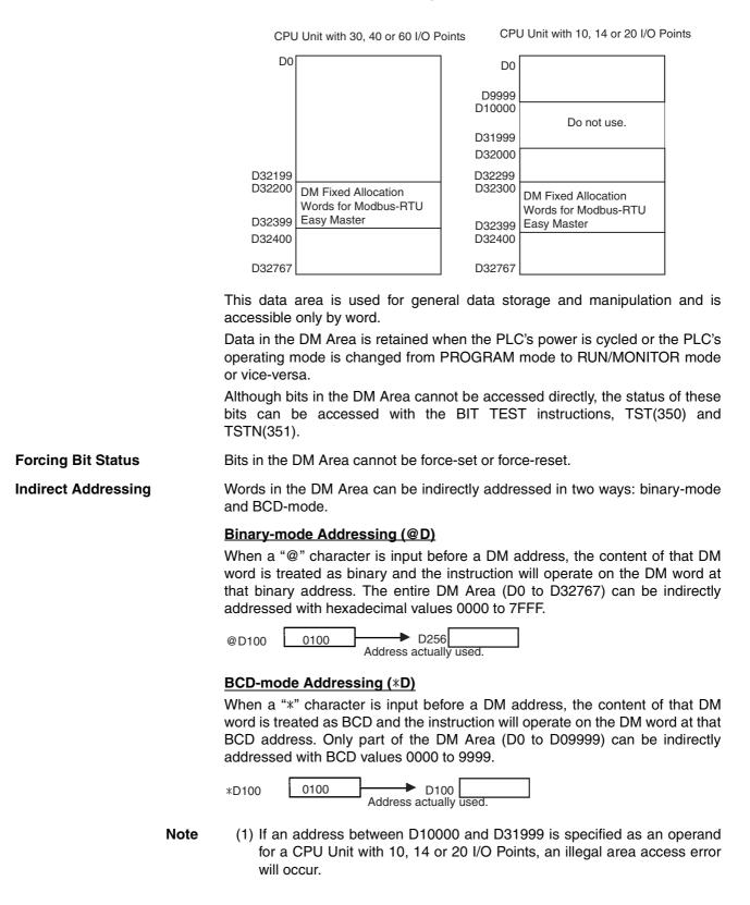
(2) If two-word data is accessed from the last address in the DM Area (D9999 for the CP1L-L\_D\_-\_ and D32767 for other CPU Units), the Access Error Flag (P\_AER) will turn ON and the data at D9999 or D32767 will not be read or written.
