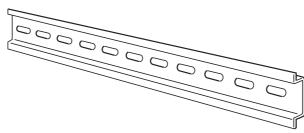
Secure the DIN Track to the control panel using M4 screws separated by 210 mm (6 holes). The tightening torque is  $1.2 \text{ N} \cdot \text{m}$ .
