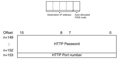
If the password for accessing the Ethernet Option Board's Web page is forgotten, find out it in this area. It is written in ASCII format.
