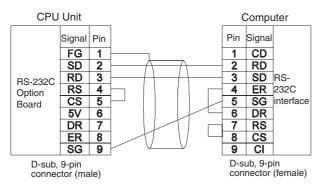
• Using NT-AL001 Converting Link Adapters
