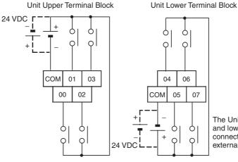
The Unit's upper terminal block COM and lower terminal block COM are connected internally, but connect them externally as well.
