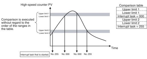
**Note** The range comparison table can be used without starting an interrupt task when the comparison condition is met. The range comparison function can be useful when you just want to know whether or not the high-speed counter PV is within a particular range.
