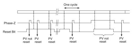
Software Reset The high-speed counter's PV is reset when the corresponding High-speed Counter Reset Bit goes from OFF to ON.
