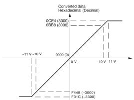
Voltage in the -10 to 10 V range corresponds to hexadecimal values F448 to 0BB8 (-3,000 to 3,000). The range of data that can be converted is F31C to 0CE4 hex (-3,300 to 3,300). A negative voltage is expressed as two's complement.
