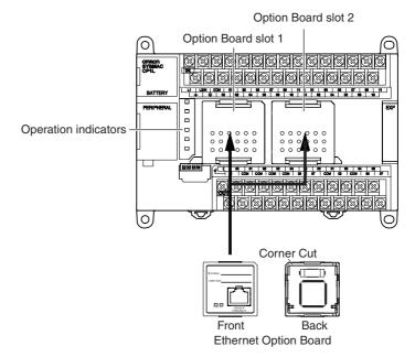
**Note** If two CP1W-CIF41 (unit version 1.0) Ethernet Option Boards are mounted on the CP1L/CP1H PLC, the CP1W-CIF41 mounted on Option Board slot1 (left side) will run in abnormal status and ERR indicator will be ON. If the ladder program operates the with CP1W-CIF41 fatal error, the PLC will generate the non-fatal error.
