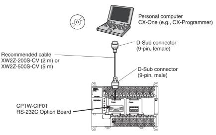
Connect the CX-Programmer to the RS-232C port of the CP1W-CIF01 Option Board by XW2Z-200S-CV/500S-CV RS-232C cable.
