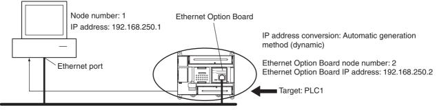
Ethernet (Network address: None) FINS/UDP method
