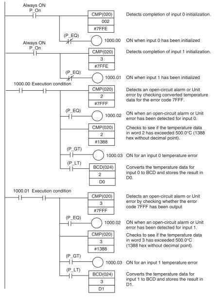
2. The following programming example shows how to convert the data for temperature input 0 to BCD and store the result in D0 and D1. "0001" is stored in D1 when the input data is a negative value. The following system configuration is used.
