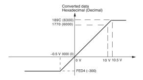
Voltage in the 0 to 10 V range corresponds to hexadecimal values 0000 to 1770 (0 to 6,000). The range of data that can be converted is FED4 to 189C hex (-300 to 6,300). A negative voltage is expressed as two's complement.
