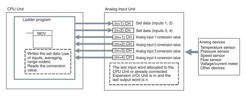
1. Connecting the Analog Input Unit
