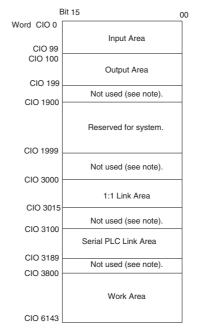
**Note** The parts of the CIO Area that are labelled "not used" may be used in programming as work bits. In the future, however, unused CIO Area bits may be used when expanding functions. Always use Work Area bits first.
