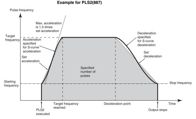
The same type of S-curve acceleration/deceleration can be used for ACC(888) as well.
