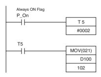
TIM 005 will start as soon as power turns ON. After 0.1 to 0.2 s (100 to 200 ms), the Completion Flag for TIM 005 will turn ON, and the data stored in DM 0100 will be moved to IR 102 as the conversion data for analog output 1.
