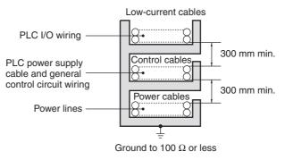
• If the I/O wiring and power cables must be placed in the same duct, they must be shielded from each other using grounded steel sheet metal.
