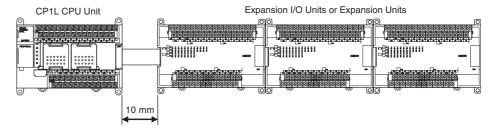
If sufficient space cannot be provided between the CPU Unit and the first Expansion Unit or Expansion I/O Unit, use the PLC in an ambient temperature of 0 to  $50^{\circ}$ C.
