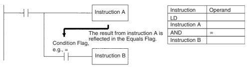
Since the Condition Flags are shared by all of the instructions, program operation can be changed from its expected course by interruption of a single task. Be sure to consider the effects of interrupts when writing the program. Refer to *SECTION 2 Programming* of *CS/CJ Series Programming Manual* (W394) for more details.
