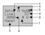
Press the **OK** button to enter the User Monitor Setup Screen. The final digit of the Screen No. will be flashing.
