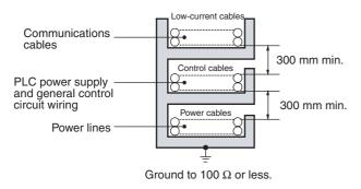
• If the I/O wiring and power cables must be placed in the same duct, they must be shielded from each other using grounded steel sheet metal.
