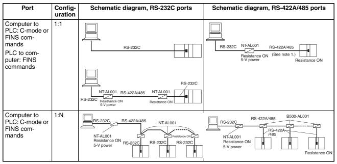
Note (1) Four-wire connections must be used for RS-422A/485 connections with Host Link communications.
