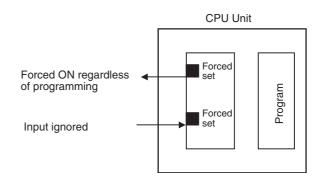
The following areas can be force-set and reset: CIO Area, Work Area, Timer Completion Flags, HR Area, Counter Completion Flags.
