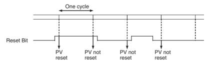
**Note** The comparison operation can be set to stop or continue when a high-speed counter is reset. This enables applications where the comparison operation can be restarted from a counter PV of 0 when the counter is reset.
