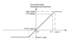
Voltage in the 0 to 5 V range corresponds to hexadecimal values 0000 to 1770 (0 to 6,000). The range of data that can be converted is FED4 to 189C hex (-300 to 6,300). A negative voltage is expressed as two's complement.
