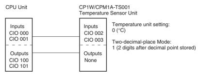
In this example, 100 times the temperature data for temperature input 0 is stored in binary form in D100 to D102.
