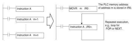
If, for example, instruction A above is a comparison instruction, table data could be read from start to the end of the table to compare all of the data with a specific value. In this way, blocks of user-defined processing can be freely created depending by applying Index Registers.
