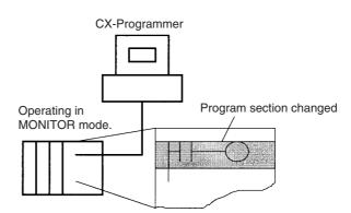
The cycle time will be increased by from one to several cycle times if the program in the CPU Unit is edited online in MONITOR mode. The cycle time will also be increased to back up data in the flash memory after online editing. The BKUP indicator will be lit during this period and the progress of the backup will be displayed on the CX-Programmer. The increases per cycle are listed in the following table.
