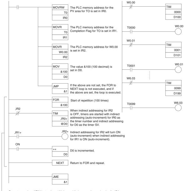
Repeat execution of TIM instructions 100 times while incrementing each value for IR0 (timer number, PV), IR1 (Completion Flag), IR2 (W0.00 on), and @D0, and start T0 to T99.
