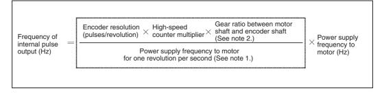
Note (1) Calculate the power supply frequency for one revolution per second from the motor specifications. For example, with a 1,800-r/min (60-Hz) motor (30 r/s), the power supply frequency for one revolution per second would be calculated as follows: 60 [Hz] ÷ 30 [r/s] = 2 [Hz].
