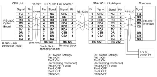
Note We recommend using the following NT-AL001 Link Adapter Connecting Cables to connect to NT-AL001 Link Adapters. XW2Z-200T-1: 2 m XW2Z-500T-1: 5 m
