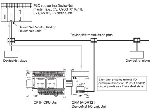
From the standpoint of the CP1L CPU Unit, the 32 input bits and 32 output bits allocated to the DeviceNet I/O Link Unit are identical to input and output bits allocated to Expansion I/O Units even though the DeviceNet I/O Link Unit does not control external inputs and outputs. The input and output bits allocated to the DeviceNet I/O Link Unit are one side of an I/O link between the slave CPU Unit and the CP1L CPU Unit to which the Master Unit is connected.
