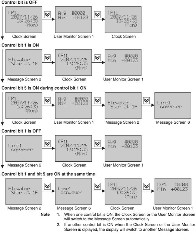
3. If another control bit is ON when one Message Screen is diplayed, the display will not change until one of the control bit is OFF.
