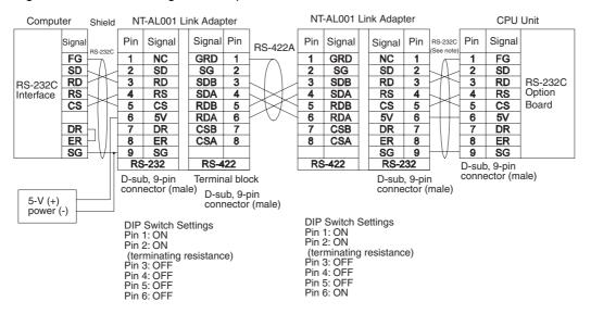
Note We recommend using the following NT-AL001 Link Adapter Connecting Cables to connect to NT-AL001 Link Adapters. XW2Z-070T-1: 0.7 m
