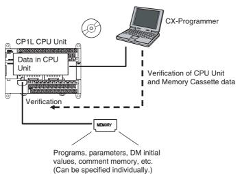
This function can be used for operations such as confirmation after data has been written to the Memory Cassette, or confirming that the data in the backup matches the data in the CPU Unit.
