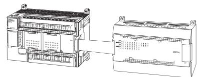
3. Replace the cover on the CPU Unit's or the Expansion I/O Unit's expansion connector.
