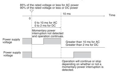
The following timing chart shows the CPU Unit power OFF operation in more detail.
