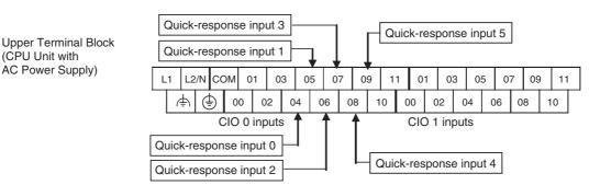
The 6 input bits CIO 0.04 to CIO 0.09 can be used as quick-response inputs.
