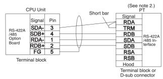
• Communications Mode: Host Link (unit number 0 only for Host Link) NT Link (1:N, N = 1 Unit only)
