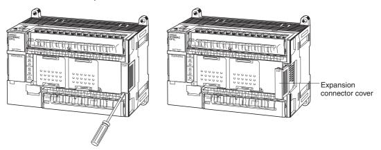
2. Insert the Expansion I/O Unit's connecting cable into the CPU Unit's or the Expansion I/O Unit's expansion connector.
