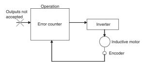
If the following settings are made in the PLC Setup, the inverter frequency command value will be calculated automatically and set in A23 in the Auxiliary Area. These settings are on the Inverter Positioning 0 Tab Page in the PLC Setup.
