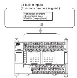
**Note** Settings in the PLC Setup determine whether each input point is to be used as a normal input, interrupt input, quick-response input, or high-speed counter.
