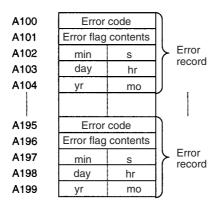
The following data would be generated in an error record if a memory error (error code 80F1) occurred on 1 April 1998 at 17:10:30 with the error located in the PLC Setup (04 hex).
