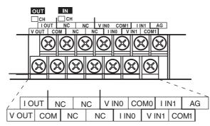
Note For current inputs, short V IN0 to I IN0 and V IN1 to I IN1.
