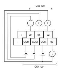
AC-power-supply models have a 24-VDC output terminals (+/-) on the lower terminal block. They can be used as a DC power supply for the input circuit.
