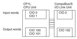
The input word (m+1) contains the 8 bits of data from the Master Unit and two CompoBus/S communications flags.
