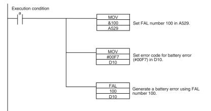
**Note** Use the same methods as for actual system errors to clear the simulated system errors. Refer to the *11-2 Troubleshooting* for details. All system errors simulated with FAL(006) and FALS(007) can be cleared by cycling the power supply.
