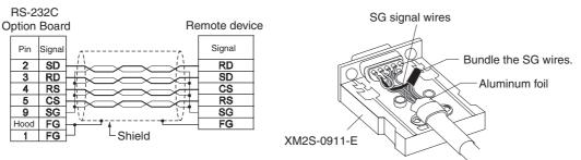
**Note** The Hood (FG) is internally connected to the ground terminal (GR) on the CPU Unit. Therefore, FG is grounded by grounding the ground terminal (GR) on the power supply terminal block. Although there is conductivity between the Hood (FG) and pin 1 (FG), connect the Hood (FG) to the shield because the Hood (FG) has smaller contact resistance with the shield than pin 1 (FG), and thus provides better noise
