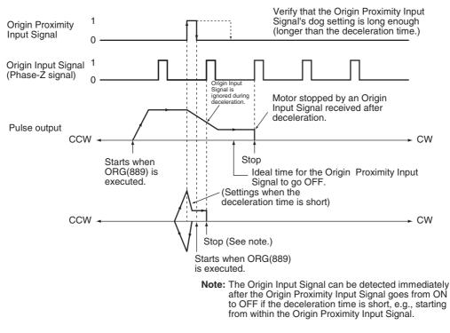
a Origin Proximity Input Signal dog setting that is long enough (longer than the deceleration time.)
