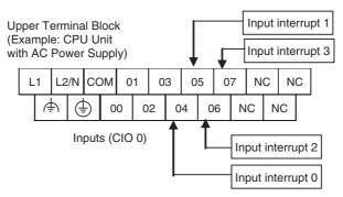
Input Terminal Block of CPU Units with 20 I/O Points The 6 input bits CIO 0.04 to CIO 0.09 can be used for input interrupts.
