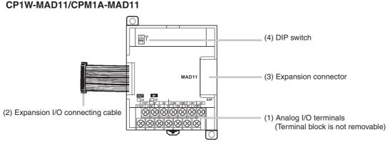
(1) Analog I/O Terminals Connected to analog I/O devices.
