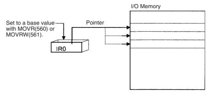
**Note** (1) It is possible to specify regions outside of I/O memory and generate an Illegal Access Error when indirectly addressing memory with Index Registers. Refer to *Appendix E Memory Map* for details on the limits of PLC memory addresses.
