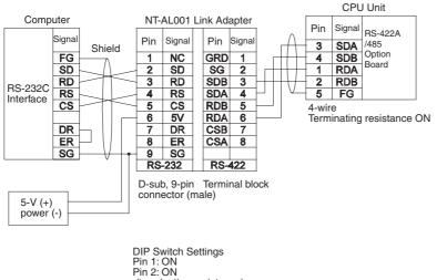
Pin 1: ON Pin 2: ON (terminating resistance) Pin 3: OFF Pin 4: OFF Pin 5: OFF Pin 6: OFF
