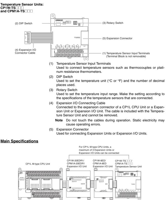
Thermocouples or platinum resistance thermometers
