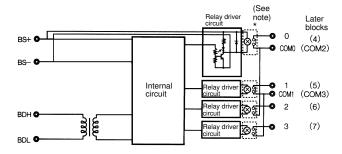
**Note:** The G3DZ-2R6PL Power MOS FET Relay is inserted into this portion of the SRT1-R0F08 and SRT2-R0F16.
