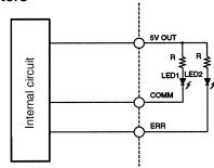
R: LED current limiting resistor LED1: LED for COMM
