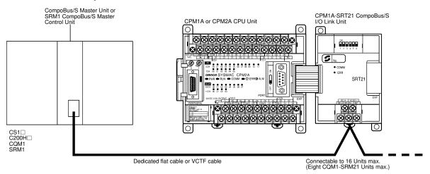
Note: A single CompoBus/S I/O Link Unit together with a maximum of two other Expansion I/O Units can be connected to the CPM1A or CPM2A CPU Unit.
