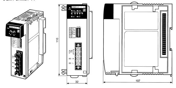
**Note:** Refer to the *CQM1 Operation Manual* for details on the dimensions when the Master Unit is installed in the PC's Backplane.
