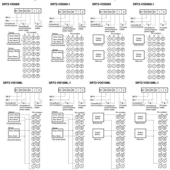
Note: 1. V terminals and G terminals are respectively connected internally.
