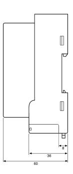
The above dimensions apply to the SRM1-C02-V2. The SRM-C01-V2 has no RS-232C port.
