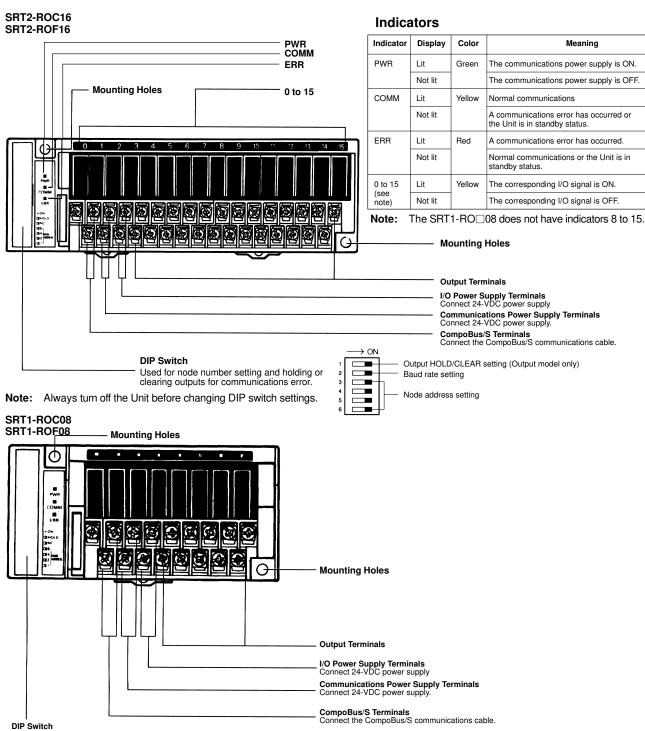
Used for node number setting and holding or clearing outputs for communications error.
