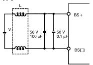
L: Coil for the common mode Install the coil near the SRT1.
