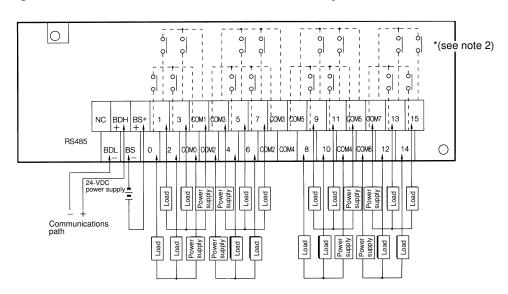
Note: 1. Dotted lines indicate internal connections. SRT1-ROC08 and SRT1-ROF08 have the 0 to 7 and COM0 to COM3 terminals only.
