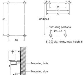
The D4BS can be mounted more securely by adding two protruding portions, each of which is 5 mm maximum in height and  $5^{-0.05}/_{-0.15}$  mm in diameter as shown below.
