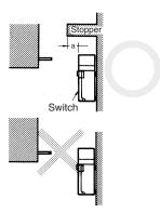
Refer to *Dimensions* for the mounting dimension of the Operation Key and mount the Operation Key correctly. The Operation Key will soon become damaged or worn out if it is not mounted correctly.
