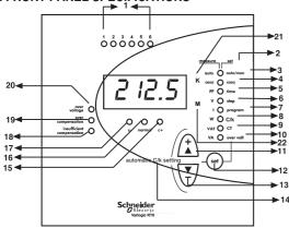
On the front panel of RT6, there are warning LEDs, display and 3 buttons for settings.
