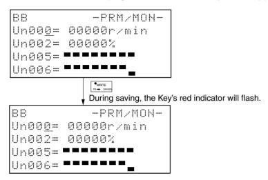
**Note** Do not turn OFF the Servo Driver control power supply during the saving process. Doing so will prevent the screen from being saved. If the screen has not been saved successfully, the previous default setting will be used, but no alarm will occur.
