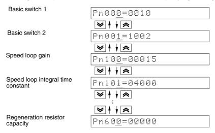
• When the cursor is on the right side (the setting data side), pressing the Up and Down Keys increments or decrements the numeric value of the digit at the cursor.
