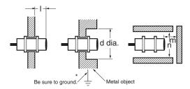
\* Be sure to ground the metal object, otherwise Sensor operation will not be
