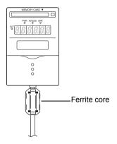
1 Attach the ferrite core (supplied) to the Data Storage Unit's I/O cable.
