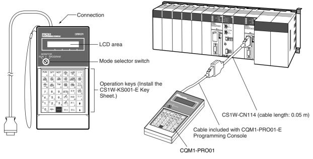
Connect the CPU Unit to the Programming Console with the following cables. CS1W-CN114 (Cable length: 0.05 m)
