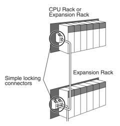
The connectors can be inserted only one way; they cannot be inserted upside down. Be sure that the connectors fit properly as they are inserted.
