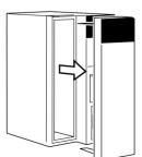
3. Align the Inner Board with the groove and slide it into the compartment.
