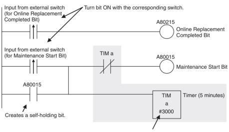
If the Maintenance Start Bit is turned ON by mistake, an error will not be generated even if a Unit fails. Therefore, the Maintenance Start Bit is turned OFF after a short time. (In this example, it is turned OFF by the 5-minute timer.)
