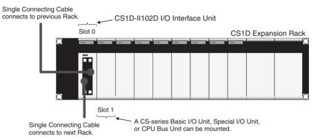
If a CS1D I/O Interface Unit is mounted in slot 1 only, a Basic I/O Unit, Special I/O Unit, or CPU Bus Unit cannot be mounted in slot 0.
