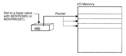
**Note** It is possible to specify regions outside of I/O memory and generate an Illegal Access Error when indirectly addressing memory with Index Registers. Refer to *Appendix E Memory Map* for details on the limits of PLC memory addresses.
