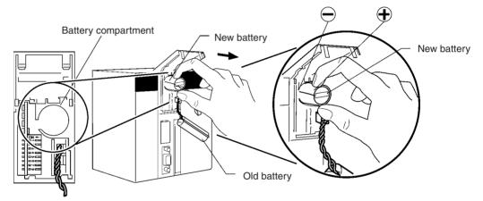
5. With the old battery connected, insert the new battery's connector in the open connector in the CPU Unit. Be sure that the connector is inserted so that its red wire is at the top and the white wire is at the bottom.
