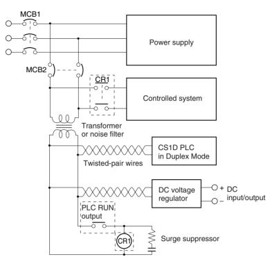
**Note** Do not latch the RUN output and use it in a circuit to stop a controlled object. Chattering of the relay contacts used in the output may cause incorrect operation.
