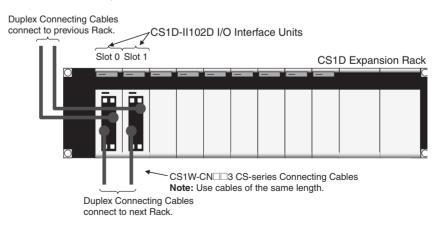
**Note** 1. When using duplex Connecting Cables, always use cables that are the same length.
