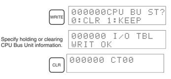
**Note** If an error occurs when creating the I/O tales, detailed I/O table error information is stored in A261 whenever the I/O tables. This information can be used to identify the Unit causing the error.
