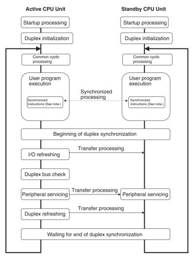
Note These instructions include IORF(097) (I/O REFRESH), DLINK(226) (CPU BUS UNIT I/O REFRESH), IORD(222) (INTELLIGENT I/O READ), IOWR(223) (INTELLIGENT I/O WRITE), PID(190) (PID), RXD(235) (RECEIVE), FREAD(700) (READ DATA FILE), and FWRIT(701) (WRITE DATA FILE).
