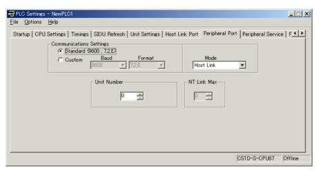
With a Duplex CPU System, these settings are valid when the PRPHL pin on the DIP switch on the Duplex Unit is turned ON.
