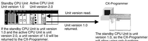
will allow using only functions supported by unit version 1.0. the unit version when going online with the PLC setting windows, such as the PLC Setup Window.
