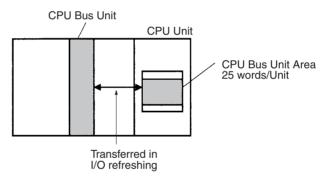
Note With CS1-H CPU Units, the CPU BUS I/O REFRESH instruction (DLNK(226)) can be executed in the ladder program to refresh the CIO Area words allocated to the CPU Bus Unit of a specified unit number.
