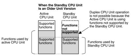
A31708 will turn ON to indicate a CPU Unit Version Verification Error as the cause of the Duplex Verification Error. This error will be detected at the following times.
