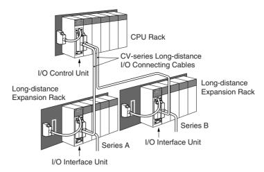
The connecting port for each CV-series Long-distance I/O Connecting Cable depends on the system configuration and the Rack being connected, as shown in the following diagrams. The PLC will not operate properly if the Racks are not connected as shown in the following diagrams.
