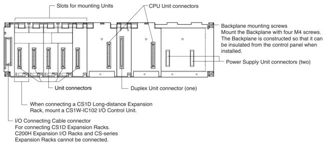
**Note** Backplanes produced from July 2005 have screw holes that allow an Expansion Rack Cable Mounting Bracket to be attached to secure the cable.
