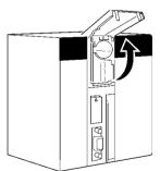
3. Remove the old battery from the compartment, but leave its connector connected.
