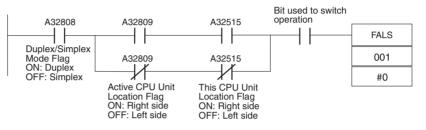
**Note** If the right and left CPU Units are made to perform different operation, they will not longer be synchronized and a duplex bus error or other error may occur. Do not use the above type of programming with A32515 (This CPU Unit Location Flag) for any other application.
