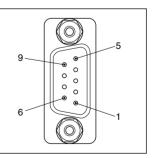
**Note** Do not use the 5-V power from pin 6 of the RS-232C port for anything but an NT-AL001 Link Adapter or CJ1W-CIF11 Conversion Adapter. Using this power supply for any other external device may damage the CPU Unit or external devices.
