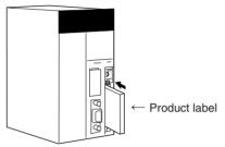
3. Push the Memory Card securely into the compartment. If the Memory Card is inserted correctly, the Memory Card eject button will be pushed out.
