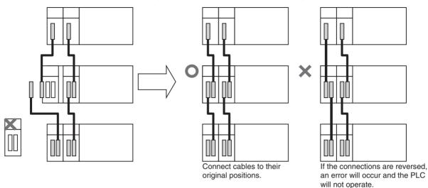
4. Verify that the Expansion Units RDY Indicator is lit and its ERR Indicator is not lit. If there are no errors, the Unit replacement is completed.
