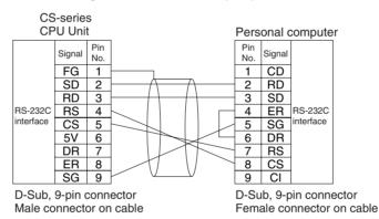
Use the following connectors and cables when creating RS-232C cable for connecting to the RS-232C port.
