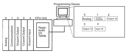
The I/O Verification Error Flag (A40209) will be turned ON if the models and locations of the Units actually mounted to the PLC (CPU Rack and Expansion I/O Racks) do not match the information in the Registered I/O Tables.
