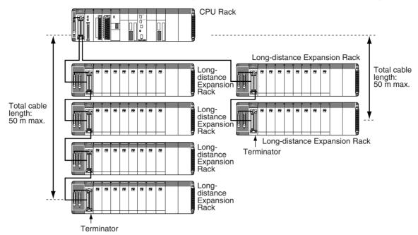
Example 2: Long-distance Expansion Rack I/O Connecting Cables
