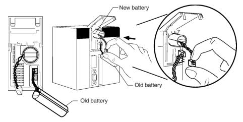
6. Remove the old battery's connector.
