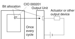
Immediate Refreshing (Single CPU Systems Only) When the immediate refreshing variation of an instruction is specified by inputting an exclamation point just before the instruction, and the instruction's operand is an output bit or word, the content of the word containing the bit or the word itself will be output just after the instruction is executed. This immediate refreshing is performed in addition to the normal I/O refreshing performed once each cycle.
