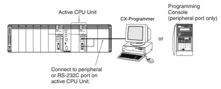
**Note** With a Duplex CPU System, operations, such as generating I/O tables and transferring the program, will not be possible if the Programming Device is connected to the standby CPU Unit.
