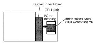
The function of the 100 words in the Inner Board Area depends upon the Duplex Inner Board being used. For details, refer to the Board's Operation Manual.
