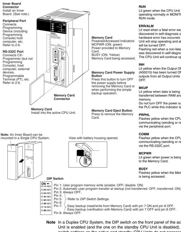
Lit green when the CPU Unit is operating normally in MONITOR or
