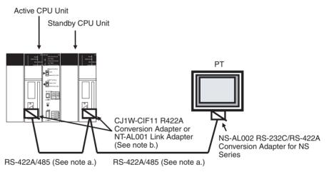
Note a) Use shielded twisted-pair cable for the RS422A/RS-485 cable.
