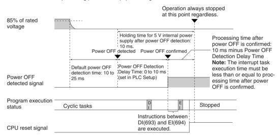
If A530 is not set to A5A5 hex, i.e., if prohibiting power interruption processing is not enabled, only the current instruction will be executed and then power interruption processing will be performed.
