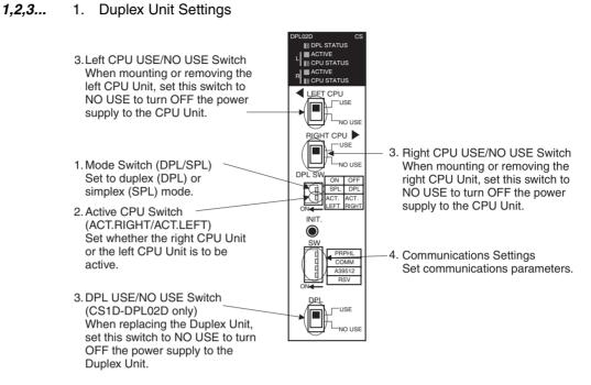
a) Set the mode switch on the Duplex Unit to DPL (duplex).
