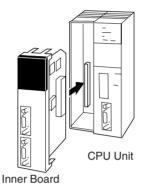
*1,2,3...* 1. Press the catches at the top and bottom of the Inner Board compartment cover and pull the cover forward.
