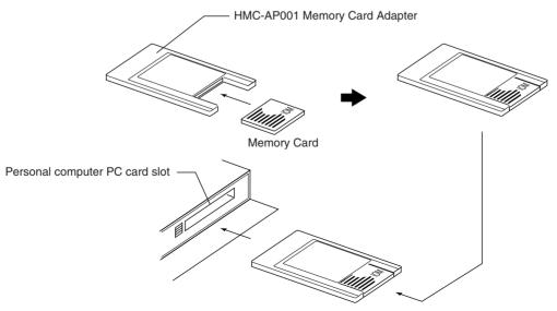
**Note** When a Memory Card is inserted into a computer using a Memory Card Adapter, it can be used as a standard storage device, like a floppy disk or hard disk.
