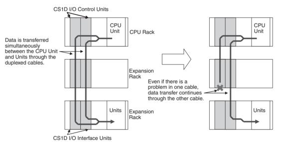
A duplex Connecting Cable system can be configured by mounting two CS1D I/O Control Units in the CPU Rack, mounting two CS1D I/O Interface Units in each Expansion Rack, and connecting the Racks with two Connecting Cables. In a PLC system with duplex Connecting Cables, data is simultaneously transferred over both cables between the CPU Unit and Units in the Expansion Racks.
