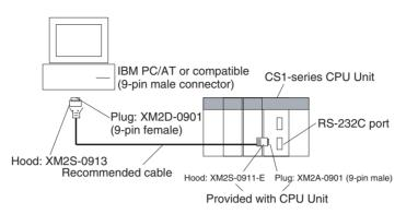
**Note** Use the special cables provided from OMRON for all connections whenever possible. If cables are produced in-house, be sure they are wired correctly. External devices and the CPU Unit may be damaged if general purpose (e.g., computer to modem) cables are used or if wiring is not correct.
