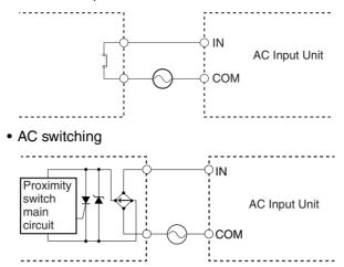
**Note** When using a reed switch as the input contact for an AC Input Unit, use a switch with an allowable current of 1 A or greater. If Reed switches with smaller allowable currents are used, the contacts may fuse due to surge currents.
