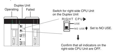
3. Replace the faulty CPU Unit with a new CPU Unit.
