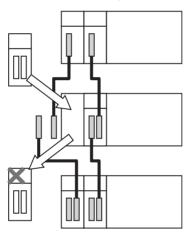
**Note** When removing and mounting a Unit, move the Unit smoothly so that it is not disconnected/reconnected repeatedly. After mounting a Unit, secure it by tightening the mounting screws to the proper torque.
