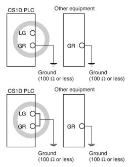
• Do not share the PLC's ground with other equipment or ground the PLC to the metal structure of a building. The configuration shown in the following diagram may worsen operation.
