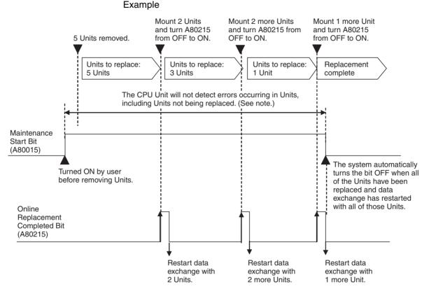
**Note** If you want to detect errors in other Units before all of the Units have been replaced online, turn OFF the Maintenance Start Bit.
