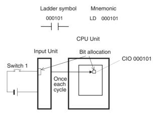
Immediate Refreshing (Single CPU Systems Only) When the immediate refreshing variation of an instruction is specified by inputting an exclamation point just before the instruction, and the instruction's operand is an input bit or word, the word containing the bit or the word itself will be refreshed just before the instruction is executed. This immediate refreshing is performed in addition to the normal I/O refreshing performed once each cycle.
