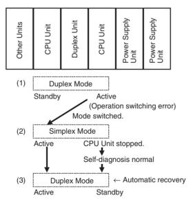
In order for automatic recovery to be enabled, the power to the other CPU Unit must not be OFF and the Mode Setting Switch must be set to DPL. If the mode cannot be automatically returned to Duplex Mode, the following bits in the Auxiliary Area (CPU Unit Duplex Unit Recovery Flags) will turn ON.
