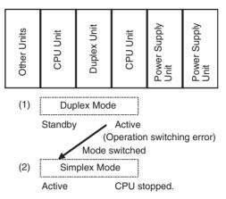
The CPU Unit where the error occurred can be replaced while the system continues operating using the CPU Unit online replacement function.
