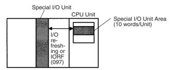
Each Special I/O Unit is allocated 25 words based on its unit number, as shown in the following table.
