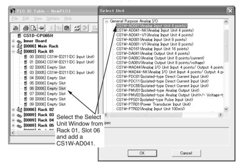
Select *Options - Online Add Unit - reflection*. The Unit addition will be completed if the Unit selected in the CX-Programmer matches the Unit that was actually added.
