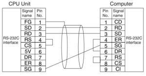
D-sub, 9-pin connector (male) D-sub, 9-pin connector (female)
