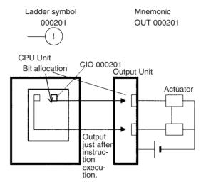
**IORF(097) Refreshing** When IORF(097) (I/O REFRESH) is executed, the ON/OFF status of output bits in the specified range of words is output to their external devices. This I/O refreshing is performed in addition to the normal I/O refreshing performed once each cycle.
