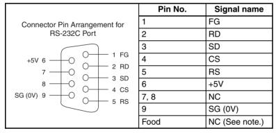
Note The hold will be the same electrical potential as the connector hood on the other end of the cable.
