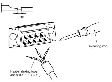
4. Move the heat-shrinking tubes onto the soldered area and shrink them into place.
