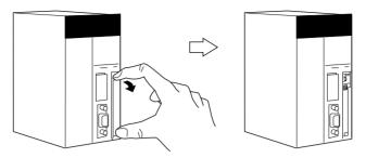
2. Insert the Memory Card with the label facing to the right. (Insert with the  $\Delta$  on the Memory Card label and the  $\triangleleft$  on the CPU Unit facing each other.)
