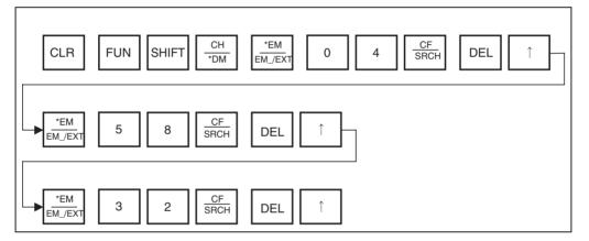
Ending Replacement of Multiple Units When the last Unit has been replaced and the online replacement procedure for it has been completed, the replacement procedures for the remaining Units can be ended either by pressing the CLR Key and then performing steps *1*. through *3*. and then step *7*. in the basic procedure, or by using the following procedure to end the replacement procedures directly using step *7*.
