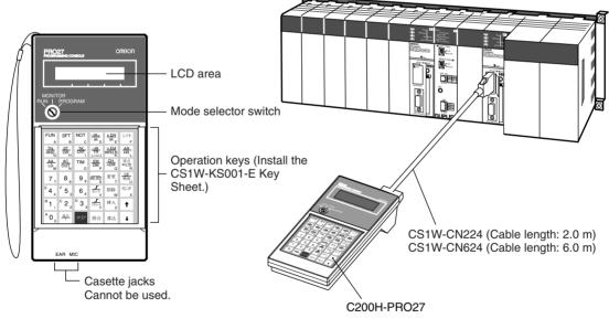
Connect the CPU Unit to the Programming Console with the following cables. CS1W-CN224 (Cable length: 2.0 m) CS1W-CN624 (Cable length: 6.0 m)
