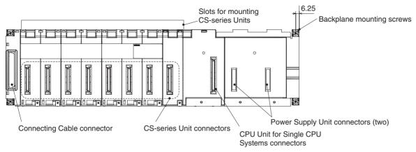
**Note** To protect unused connectors, always cover them with CV500-COV01 I/O Unit Connector Covers (sold separately) or mount the CS1W-SP001 Spacer Unit (sold separately). When using only one Power Supply Unit, cover the unused Power Supply Unit connector with a C500-COV01 Power Supply Unit Connector Covers (sold separately).
