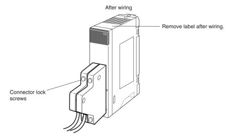
Tighten the connector-attaching screws to a torque of 0.2 N·m. The following examples show applications for preassembled OMRON Cables. Contact your OMRON dealer for more details.
