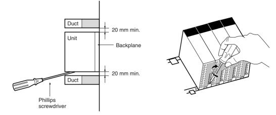
4. To remove a Unit, use a phillips-head screwdriver to loosen the screw at the bottom of the Unit, rotate the Unit upward, and remove it.
