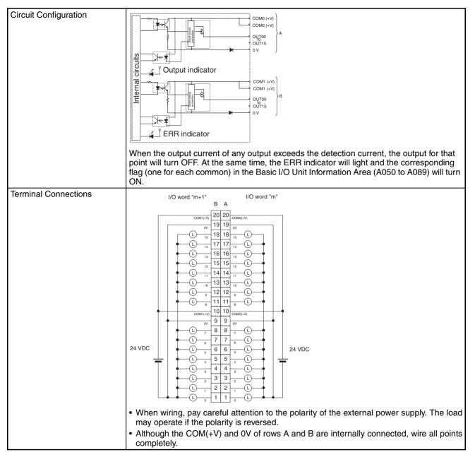
Note The maximum load currents will be 2.0 A/common and 4.0 A/Unit if a pressure-welded connector is used.
