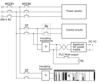
The Duplex CPU and Expansion Backplanes for a CS1D PLC support Duplex Power Supply Units. If anything happens to interrupt the power supply from one of the Power Supply Units, the other one will continue supplying power to the Unit on the Rack. To ensure that the PLC will continue operating even if the power supply to the Power Supply Unit is interrupts, always provide power to two Duplex Power Supply Units from different power sources.
