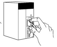
Hold the grips on the side of the connector and push into the port.
