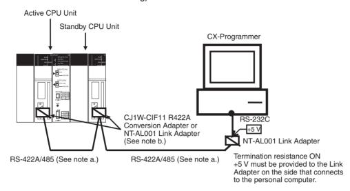
Note a) Use shielded twisted-pair cable for the RS422A/RS-485 cable.
