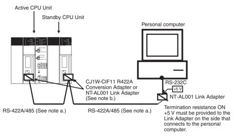
Note a) Use shielded twisted-pair cable for the RS422A/RS-485 cable.
