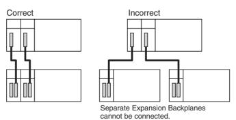
If a CS1D I/O Control Unit is mounted in slot 0 only, a Basic I/O Unit, Special I/O Unit, or CPU Bus Unit can be mounted in slot 1.
