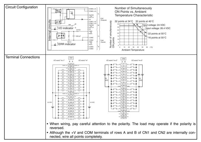
Note The ON response time will be 20 μs maximum and OFF response time will be 300 μs maximum even if the response times are set to 0 ms due to internal element delays.
