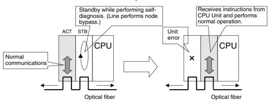
Active/standby communications have been supported since the first CS1D CPU Units were released, so they can be used on any CS1D CPU Unit (including Pre-Ver. 1.1 CPU Units). CX-Programmer version 3.1 or higher is required to make settings for duplex operation.
