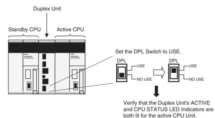
5. Verify that the new Duplex Unit's Duplex Setting Switches (DPL SW) are set to DPL, and press the Initial (INIT) Button. When the Initial Button is pressed, the DPL STATUS and CPU STATUS Indicators flash green and then stay lit when operation restarts in Duplex Mode.
