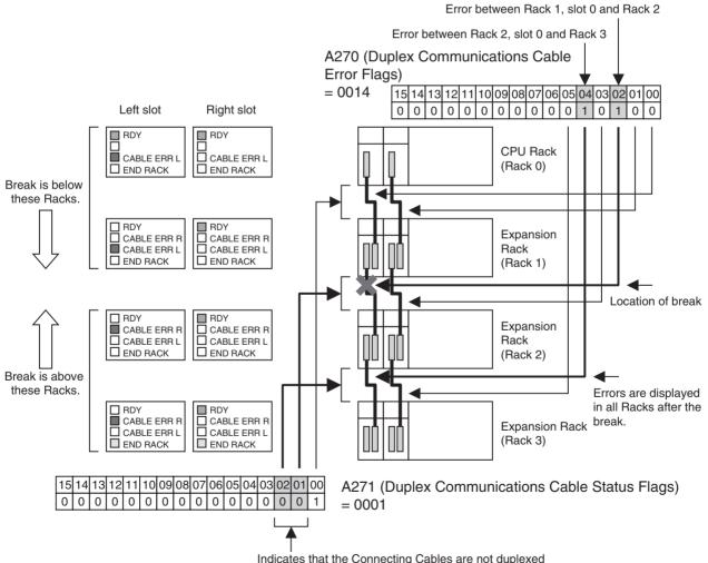
Indicates that the Connecting Cables are not duplexed between Rack 1 and Rack 2, and between Rack 2 and Rack 3.
