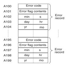
The following data would be generated in an error record if a memory error (error code 80F1) occurred on 1 April 2002 at 17:10:30 with the error located in the PLC Setup (04 hex).
