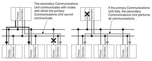
CS1D CPU Units for Duplex CPU Systems with a unit version of 1.1 or later or a CS1D CPU Unit for Single CPU Systems with a unit version of 2.0 or later is required to use Duplex Communication Units using primary/secondary communications. CX-Programmer version 2 or higher is required for duplex settings.
