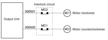
This circuit prevents outputs MC1 and MC2 from both being ON at the same time even if both CIO 000501 and CIO 000502 are both ON, so the motor is protected even if the PLC is programmed improperly or malfunctions.
