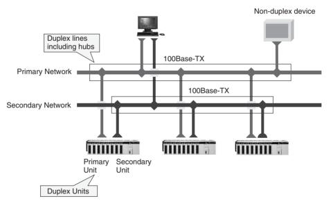
**Note** Duplex operation of Ethernet Units for a Duplex CPU System requires a CS1D CPU Unit Ver. 1.1 or later and CX-Programmer Ver. 4.0 or higher. Duplex operation of Ethernet Units for a Single CPU System is possible for any CS1D CPU Unit for Single CPU Systems, but CX-Programmer Ver. 4.0 or higher is required.
