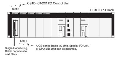
If a CS1D I/O Control Unit is mounted in slot 1 only, a Basic I/O Unit, Special I/O Unit, or CPU Bus Unit cannot used in slot 0.
