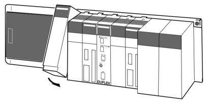
3. For a Single CPU System, install an Inner Board in the CPU Unit if required.
