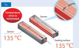
Cause not perfect sensor location there is 5°C difference vs temperature sealing surface.
