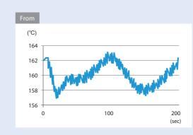
When sensor is placed closer to sealing surface, sometimes periodic temperature variation is caused by the heat on and off switching during the sealing period.
