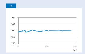
The "Automatic filter adjustment function" suppress automatically this phenomenon guarantee stable temperature control.
