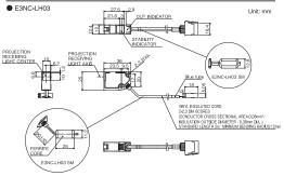
Ferrite core is mounted only E3NC-LH03 5M
