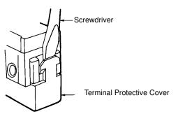
When mounting the Terminal Protective Cover to the case, align the cover on the case and then press the cover down to mount it firmly. If the cover is pressed down in an inclined position, rubber packing will deform and thus affect the sealing capability.
