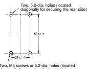
Two, M5 screws or 5.2-dia. holes (located diagonally for securing the front side)
