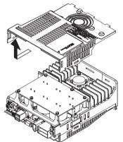
4. Remove the six mounting screws.
