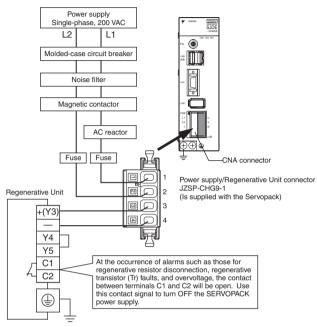
Note: 1. Pull lightly on the wires to confirm that they are securely connected.
