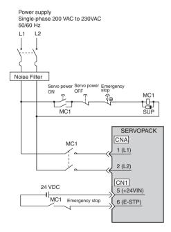
Set the following parameter to disable the emergency stop input signal if it is absolutely necessary.
