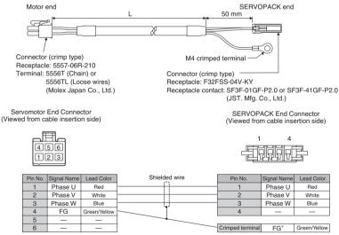
\*: Connect the FG pin to the grounding terminal of the SERVOPACK.
