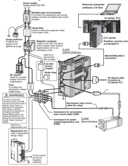
\* 1. Prepare a 24-VDC power supply for the brake separately from the sequence power supply.
