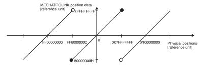
The position data is 0 when the power supply is turned ON.
