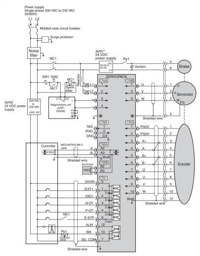
Note: 1. AVR1:24 VDC power supply for brake
