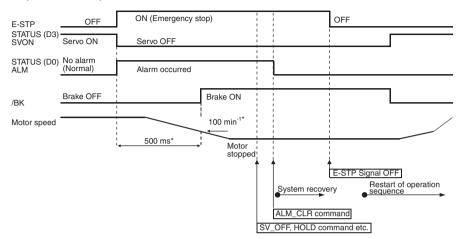
\* /BK signal is output when the motor speed reaches 100 min<sup>-1</sup> or when 500 ms elapses after the servo turns OFF.
