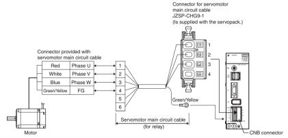
Note: Confirm pin numbers on the connector as well.
