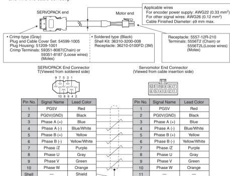
Note: Confirm pin numbers on the connector as well.
