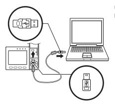
Use a USB cable (ZFX-XUSB) to connect the Controller to the PC.
