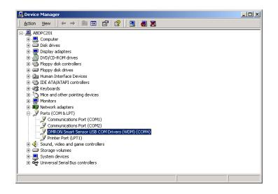
**3.** Open [Port COM/LPT], and check the COM number in [OMRON Smart Sensor USB COM Drivers (WDM) (COMxx)].
