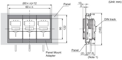
Note 1: Dimensions are shown for a panel thickness of 2.0 mm.
