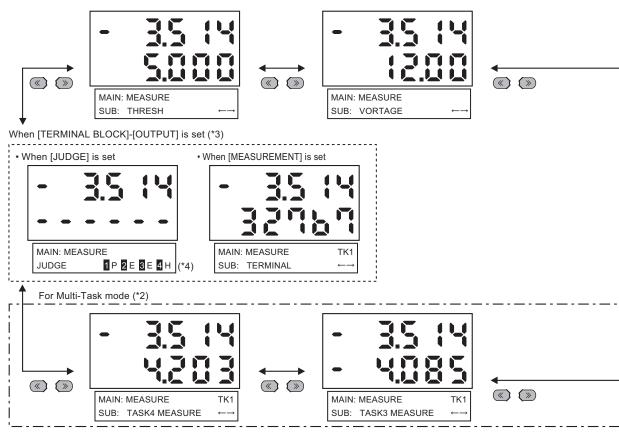
\*1) TKx on the LCD screen indicates that the measured value of the current TASKx is displayed in the main display. Switch TASK that is displayed in the main display by using the function keys.
