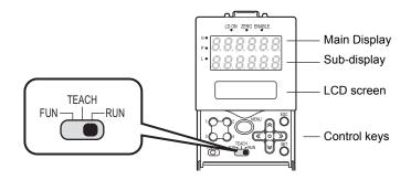
In this mode, measured values are displayed on the main display, and threshold values and other information are displayed on the sub-display.
