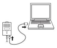
RS-232C Cable for Connecting to Programmable Controller/ Programmable Terminal
