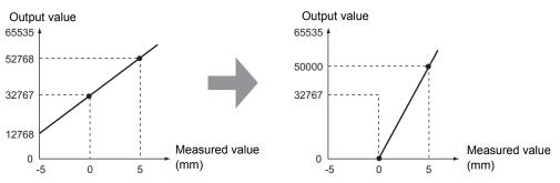
Separate the two specified points by at least 1 % of the rated measurement range for the connected Sensor Head.
