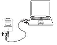
"Detected new hardware" will be displayed on the Windows tool bar, and the [New Hardware Detection Wizard] dialog box will appear.
