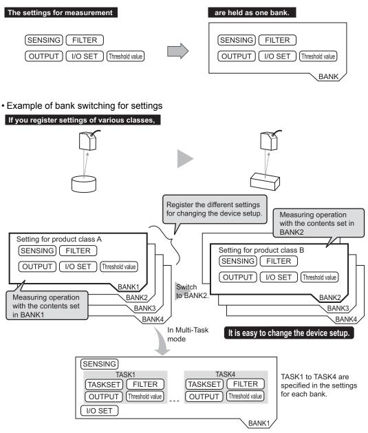
If only the "threshold value" is different in the settings for a bank, by changing the mode of the bank, you can increase the number of banks from 4 to 32.
