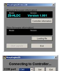
When the startup of Warp Engine ZS fails, the following screen is displayed after a message appears. Go to "Set the connection port".
