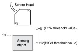
Example 3: Using zero reset to measure steps in sensing object (zero reset at each measurement)
