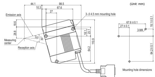
• When used in regular reflection (ZS-HLDS10)
