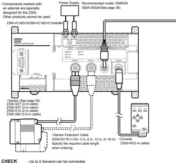
Op to 2 Sensors can be connected.
