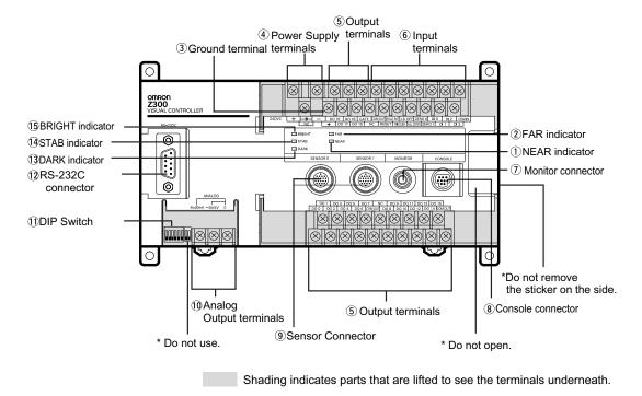
(1), (2) If the distance between the front of the Sensor and the workpiece is the measurement range, these indicators turn ON or OFF according to the distance. If the workpiece is outside the measurement range or if the light density is insufficient, both indicators will flash.
