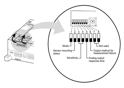
**Notice** Turn OFF the power supply before changing the DIP switch settings.
