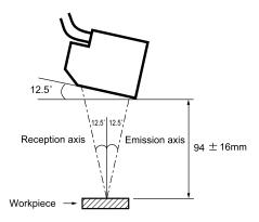
**CHECK** It is recommended that Sensor mounting is performed while monitoring the amount of received light in the menu item **Check position.** For details, refer to page 118 in the Operation Manual.
