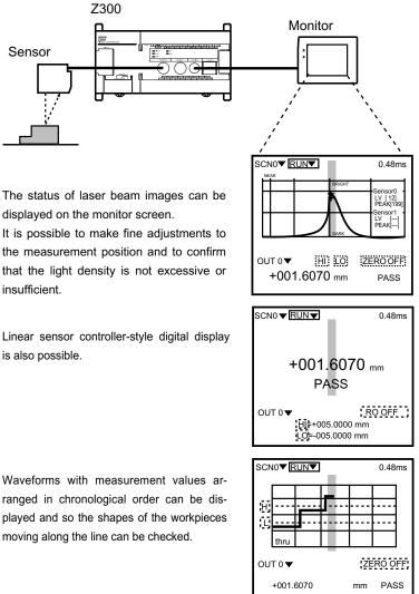
Waveforms with measurement values arranged in chronological order can be displayed and so the shapes of the workpieces
