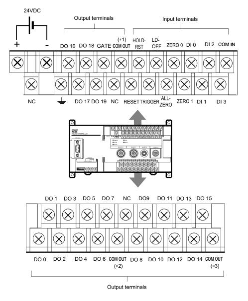
**CHECK** There are 3 types of COM OUT (\*1 to \*3) for each output terminal. Connect with reference to the table at right.
