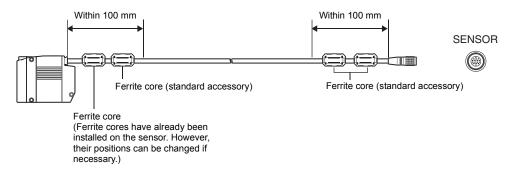
When using an extension cable, make sure that two ferrite cores are connected within 100 mm from the sensor and within 100 mm from the controller's connector, respectively.
