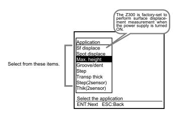
Use the **Expert Menu** to set different measurement conditions from the preset ones, or to add more detailed settings to the Application Menu settings. Refer to page 43 in the Operation Manual.
