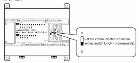
• For CPM2C (Only the RS-232C port can be connected)
