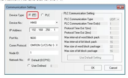
**Note** When there is CP1E PLC in the UDP network architecture, the Network No. should be 0. Otherwise, the communications through the UDP protocol between the NB and CP1E in this architecture will be impossible.
