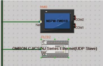
Configure the devices and set the communication parameters in the Configuration and Setup Window, then click [Add] in [PT Property] - [PT] - [Communication Setting] to set parameters for PT networkinterface communication.
