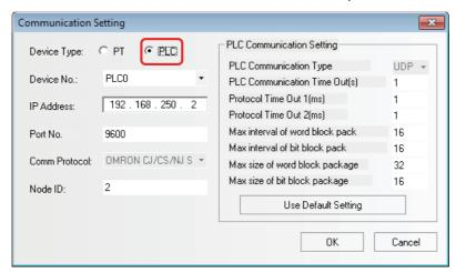
Note The settings of communication parameters should be the same as that of the actual PLC.
