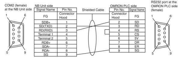
The cable for connecting the NB5Q/NB7W/NB10W Unit serial port COM2 to OMRON PLC (RS-422A)
