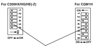
Communication condition setting for the RS-232C port Set the DIP switch 5 to OF, and activate the "settings" in PLC system settings.
