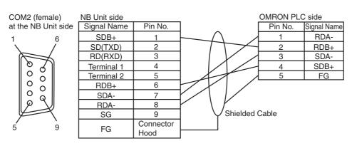
**Note** If the RS-485 connection is adopted, all needed to do is to connect the No.6 and No.8 pins and the shielded cable to the corresponding pins on the PLC side.
