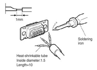
4 Pull the heat shrinkable tubes back to the soldering parts, heat them with a heat shrinking gun to make them shrink.
