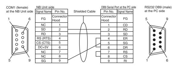
**Note** As to the 2 connection methods introduced above, the No.2, 3 and 9 pins of COM1 on the NB3Q unit side have the same definitions as those described in the above diagram, and the method for connection to a PC is also the same as above.
