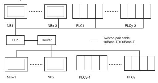
X represents the amount of NB series products, and y represents the amount of PLC. The relationship between x and y must meet the following conditions:
